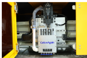
固定头重型冲孔6冲刀 Fixed heavy-duty head with 6 sizes of puncher
